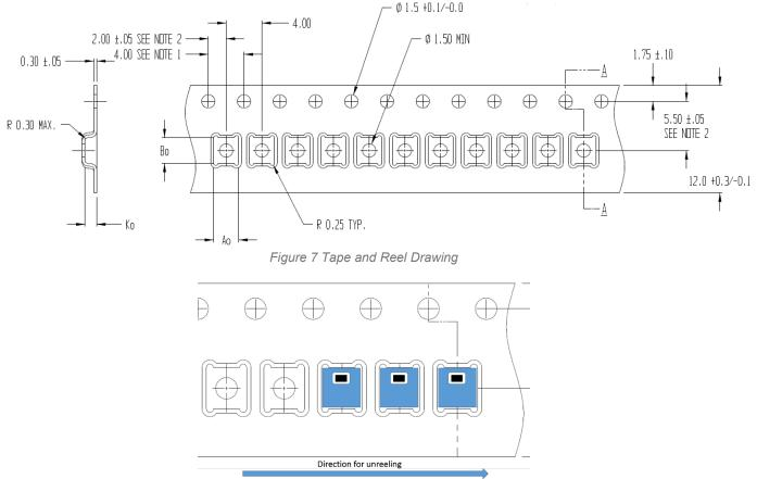
Figure 8 Product Orientation in Tape and Reel Packaging
