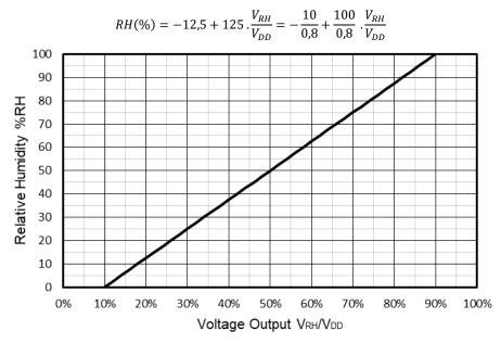
Figure 5 Relationship between ratiometric voltage output and measured relative humidity in %RH
