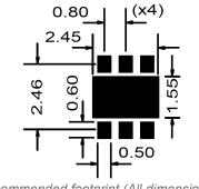
Figure 9 Recommended footprint (All dimensions are in mm)
