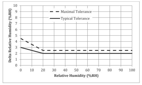
Figure 1 Humidity Sensor Rating @25°C
