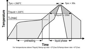
Figure 11 Reflow Soldering profile according to JEDEC standard
