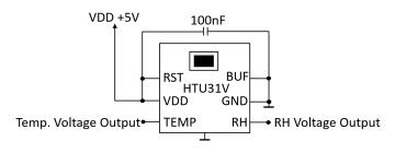
Figure 4 HTU31V Typical Application Circuit
