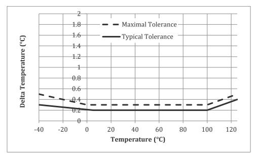
Figure 2 Temperature Sensor Rating
