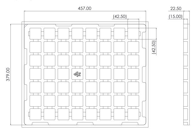
Figure 9: 56-sensor tray dimensions (in mm).
