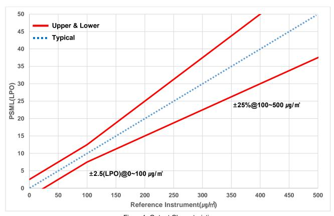
Figure 1. Output Characteristics
