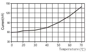
Figure 6: When VCC=3.3V, the relationship curve between typical supply current and temperature (sleep mode).Note that these data are approximately  $\pm 25\%$  off the displayed values.
