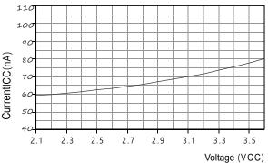
Figure 7: At a temperature of 25°C, the typical supply current is plotted against the supply voltage (sleep mode).Note that the deviation from the displayed value may be  $\pm 50\%$  of the displayed value.At 60°C, the coefficient is approximately 15(compared with Table 2)
