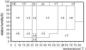
Figure 5 :The maximum error of humidity in the range of 0~80( $^{\circ}$ C),unit: (%RH)
