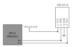
Figure 9 Typical application circuit
