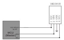
Figure 8-1 Typical Application Circuit 1, the SDA pull-up voltage and VCC are supplied by the MCU.
