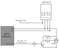
Figure 8-2 Typical Application Circuit 2,AM2301B operation is controlled by whether GND is grounded or not.
