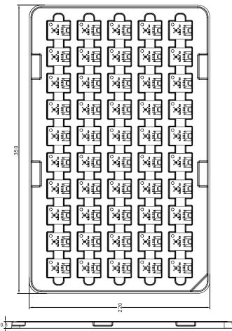
Figure 12 Location map of blister tray and sensor (unit: mm)
