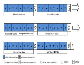
Note: The sensor needs time to collect, after the host sendsout the measurement command (0xAC), delay for more than 80 ms to read the converted data and judge whether the returned status bit is normal or not. If the status bit [Bit7] is 0, the data can be read normally, 1, the sensor is busy, the host needs to wait for the completion of data processing.
