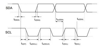
Figure 10 : Timing diagram of the digital inputs/outputs abbreviations are explained in Table 8. The thicker SDA lines are controlled by the sensor, while the regular SDA lines are controlled by the microcontroller. Note that the SDA effective read time is triggered by the falling edge of the previous conversion.
