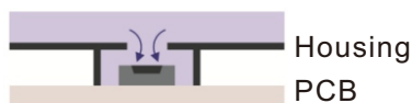
Figure 11: Suitable windows in the enclosure provide good access to environmental measurements and allow for greater air exchange.
