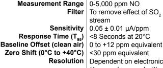
**Operating Principle** 3-electrode electrochemical 0-5,000 ppm NO Filter | To remove effect of SO, in gas stream **Sensitivity**  $0.05 \pm 0.01 \,\mu\text{A/ppm}$ <8 Seconds at 20°C <30 ppm equivalent Dependent on electronics (1 ppm when used with recommended electronics) Repeatability | 2% of signal Linearity Linear
