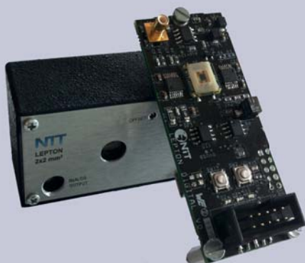
LEPTON PREAMPLIFIER WITH USB OUTPUT
