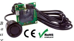
of other ultrasonic sensors. The sensors utilize a USB Micro-B connector for simple interfacing. Users can integrate many sensors into one system with little to no effect from the sensor-to-sensor interference which can occur with other ultrasonic sensor solutions. The MB8450 USB-CarSonar-WR features a True/False output and an optional range output. Deploying a network of ultrasonic sensors is simple and easy with the USB interface. \*Factory calibration and testing is standard.
