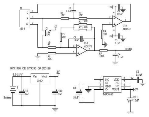
Fig2: ME4-H<sub>2</sub>S test circuit
