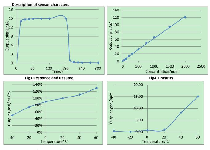
Fig5.Output of sensor at different temperature
