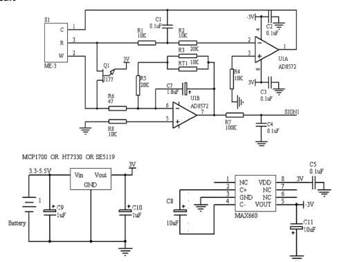
Fig2: ME4-CO test circuit
