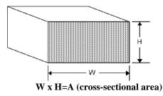
In a circular duct this cross section area equals the radius squared times  $\pi$  (3.14).
