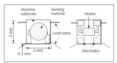
Fig 1a. Sensing element
