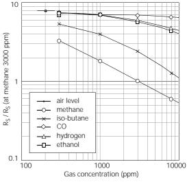
Fig 3. Sensitivity characteristics
