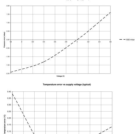
Pressure error vs supply voltage (typical)
