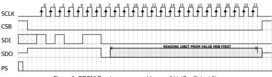
Figure 9: PROM Read sequence, address = 011 (Coefficient 3).
