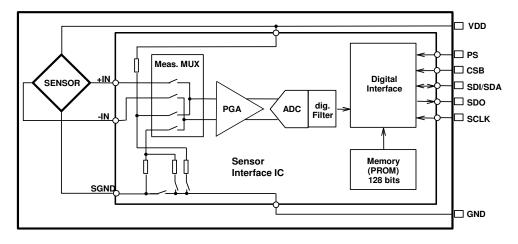
Figure 1: Block diagram of MS5607-02BA
