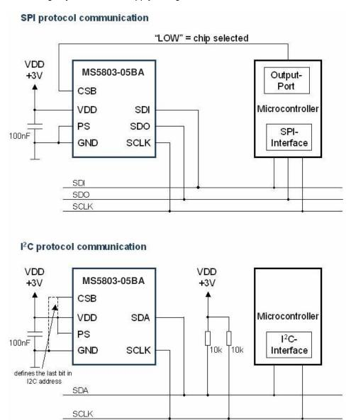
Figure 17: Typical application circuit with SPI / I<sup>2</sup>C protocol communication
