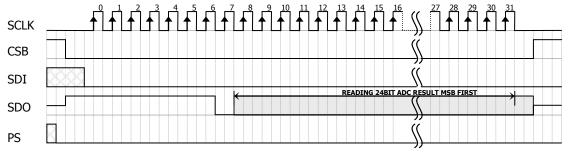
Figure 8: ADC Read sequence
