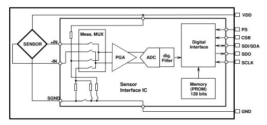
Figure 1: Block diagram of MS5803-05BA
