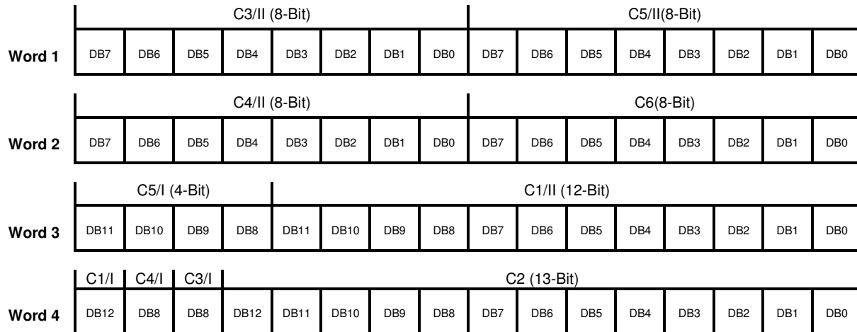
Fig. 4: Arrangement (Bit-pattern) of calibration data in Word1 to Word4
