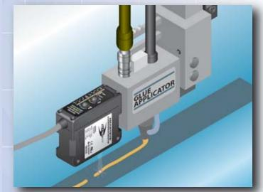
Glue Measurement for Feedback Loop
