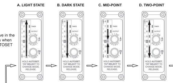
**NOTE:** LEDs move in the direction of arrows when performing an AUTOSET
