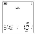
Contact detect head with the test surface vertically and press the detect head lightly, LCD displays a value, for example, 109 μm, and buzzer sounded at this time, LCD displays as shown below:
