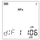
Place the sensor head to the target piece you want to measure, then press the detect head lightly to measure, the buzzer beeps, LCD will display the value of the difference between the last reading and the current reading, LCD displays as shown below:
