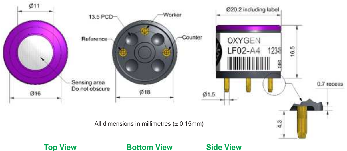
Figure 1 LFO2-A4 Schematic Diagram
