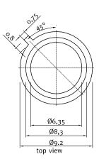
Broadband SiC based UV photodetector with integrated amplifier
