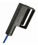
**Air Flow 2 Sensor (NO)** provides real-time recognition of air flow stoppage. This Air Flow Sensor is normally open and includes a mounting clip and clamp. Typical use is to monitor continuous air flow in an HVAC duct, under a raised floor, or near a fan on a rack cabinet or important server.
