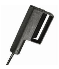
**Air Flow 1 Sensor (NC)** provides real-time recognition of air flow stoppage. This Air Movement Sensor is normally closed and includes a mounting clip and clamp. Typical use is for measuring air flow in an HVAC duct, under a raised floor, or near a fan on a rack cabinet or important server.
