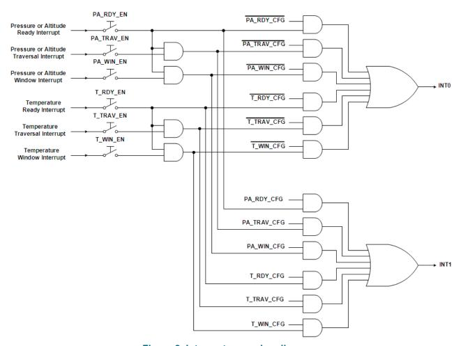
Figure 2: Interrupts mapping diagram
