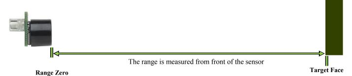
In general, the XL-MaxSonar-EZ will report the range to the leading edge of the closest detectable object. Target detection has been characterized in the sensor beam patterns.
