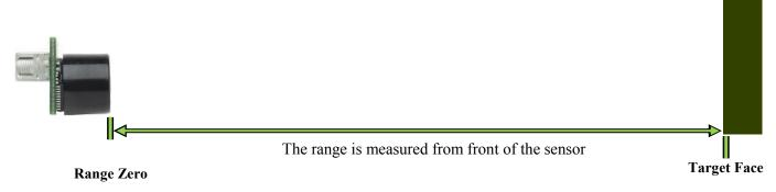
In general, the XL-MaxSonar-EZ will report the range to the leading edge of the closest detectable object. Target detection has been characterized in the sensor beam patterns.
