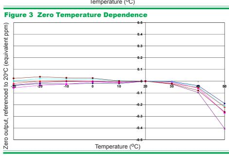
Figure 3 shows the variation in zero output caused by changes in temperature, expressed as ppm gas equivalent, referenced to zero at 20°C.
