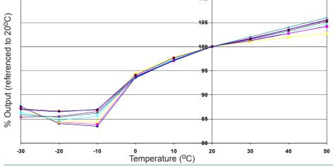
Figure 2 shows the variation in sensitivity caused by changes in temperature.
