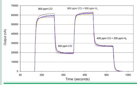
Figure 4 shows hydrogen sensitivity for a typical batch of eight CO-AX sensors at  $30^{\circ}$ C following EN50379. All sensors show less than 5% cross sensitivity when 500ppm hydrogen is added to 950ppm carbon monoxide.  $t_{90}$  is less than 45 seconds.
