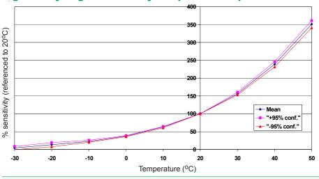
Figure 3 shows the strong temperature dependence of the CO-AX to hydrogen. Since hydrogen sensitivity is less than 4% at 20°C, hydrogen interference can practically be ignored at low temperatures. However, at 50°C hydrogen interference is 14%.
