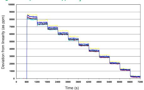
Eight PH3-B1 were tested for response from 10 to 1ppm.
