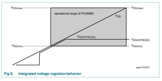
Figure 8 illustrates the behavior of the integrated voltage regulator. The gray area covers the operational range of the PCA8885. The analog part of the circuit and the switch logic is powered from  $V_{DD(INTREGD)}$ . The I<sup>2</sup>C interface and the registers are powered from  $V_{DD}$ . Therefore the I<sup>2</sup>C interface remains accessible in sleep mode, and the register values are maintained when  $V_{DD(INTREGD)}$  is powered off.
