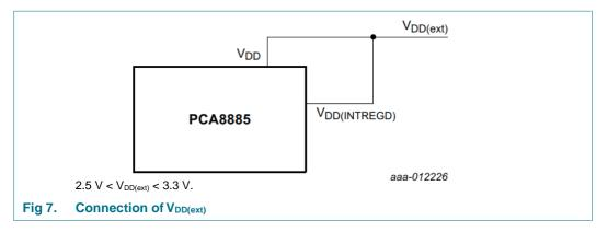
While the analog part of the circuit is powered from  $V_{DD(INTREGD)}$ , the I<sup>2</sup>C interface and the registers are powered from  $V_{DD}$ . Therefore the I<sup>2</sup>C interface remains accessible in sleep mode, and the register values are maintained when  $V_{DD(INTREGD)}$  is powered off.
