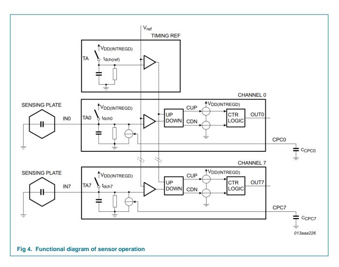
The counter following this logic counts the pulses CUP or CDN respectively. The counter is reset every time the pulse sequence changes from CUP to CDN or the other way round. The outputs OUT0 to OUT7 are only activated when 64 consecutive pulses occurred on CUP. Low-level interference or slow changes in the input capacitance do not cause the output to switch.
