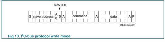
After acknowledgement, a command is sent, and after a further acknowledge a data byte is transmitted. After the last data byte, the I<sup>2</sup>C-bus master issues a STOP condition (P). Alternatively a START may be asserted to RESTART an I<sup>2</sup>C-bus access.
