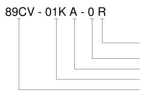
Electrical (P = Solder Pads, R = Ribbon Cable, C = Cable w/ Connector) Fitting Type Type (A = Absolute, S = Sealed Gage) Pressure Range Model
