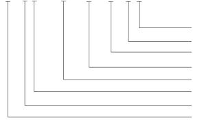
Type (G = Gage) Units (P = psi, B = Bar) Pressure Range (See Standard Ranges Table) Pressure Port (See Pressure Port Table) Specials (nnnn = Custom Drawing) Electrical Connection (1 = 2ft Cable, 2 = 4ft Cable, 4 = Packard Metri-Pack) Output (See Output Options Table) Model
