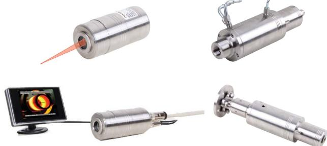
Two-Color or Ratio Pyrometers measure temperatures from the ratio of radiation signals of two adjacent wavelengths as opposed to measuring the absolute intensity within one wavelength, as with one-color pyrometers. The advantages and benefits of using two-color sensors are the following:
